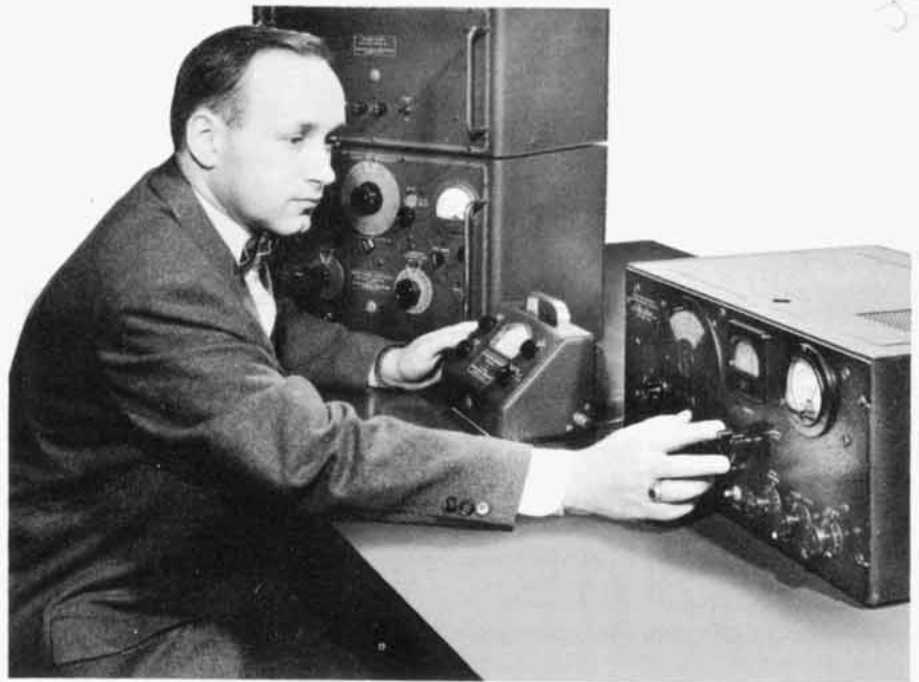
Figure 1. The author uses the 245-B to perform receiver sensitivity measurements.
